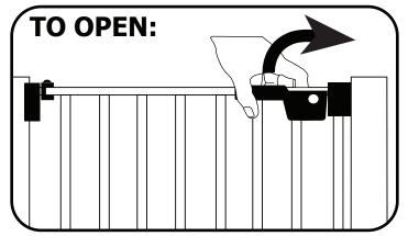
Push red safety button and lift handle  $90^{\rm o}$  upwards. Pull gate to open.
