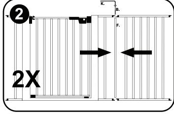
Secure upper part of rod F to gate using screw B
