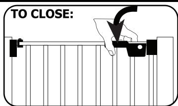
Close gate and lower handle back to original postion. Gate will click when locked.
