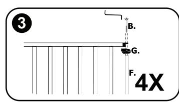
**3.** Attach end rods **F** to ends of extensions and add end caps **(E)** with long bolt **(B)**. Repeat at each corner of extensions.
