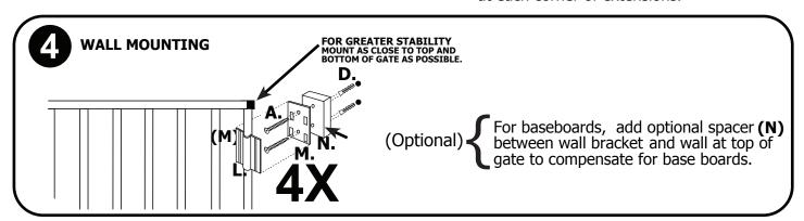
Insert screw anchor, if necessary, and attach wall bracket (M) with screw (A). Attach gate to wall with removable (L) clip (until a click sound is heard).
